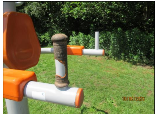
(Missing & damaged hand grips)
